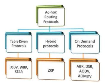
Figure 1: Routing Protocol in MANETs- An Overview
