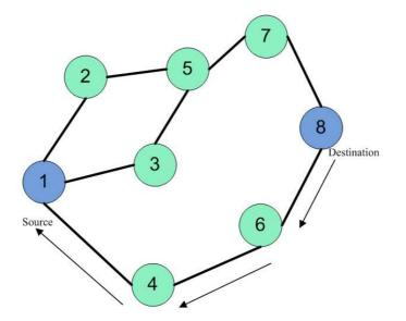
Figure 4b: Path Taken by the Route Reply (RREP) Packet
