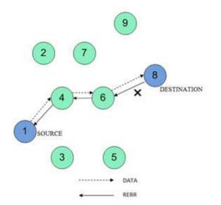
Figure 3: Route Maintenance Stage in AODV
