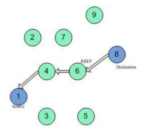
Figure 2(b): The Route Reply (RREP) Unicast for Route Discovery
